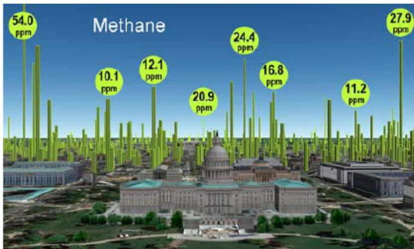
Figure 2. Natural gas leaks around Capitol Hill in Washington, D.C. From Jackson et al.<sup>28</sup>
