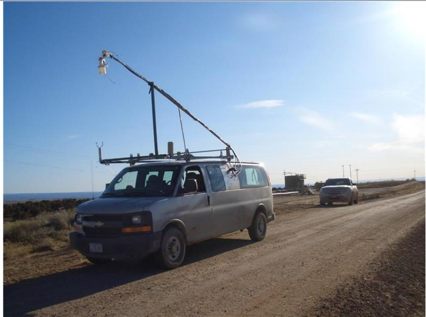
The KIT measurement instrument on board of a minivan directly measures atmospheric emissions on site with a high temporal resolution.
